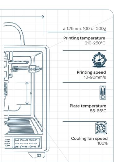
Our PLGA/HA filament is an ivory-colored filament composed of 90% PLGA and 10% hydroxyapathite\*. It is designed to resorb within 12 to 24 months after implantation. Thanks to its rigidity at room temperature, it offers exceptional stability, being above its glass transition temperature. The addition of hydroxyapatite, a natural component of bone, considerably enhances PLGA's osteoconductive properties, making it the material of choice for bone reconstruction.
