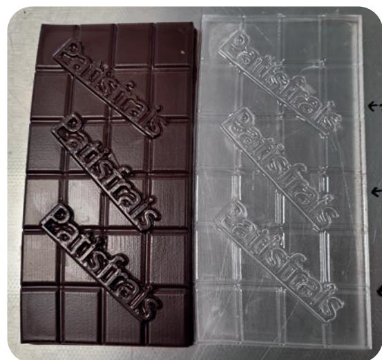
The choice of material played a key role in the success of the project. After careful consideration, we selected PETG, a polymer offering the right balance between thermal resistance, mechanical strength, and dimensional stability. This material is particularly well suited to the constraints of thermoforming, while meeting hygiene and food environment compatibility requirements, subject to regulatory approvals specific to each end use.
